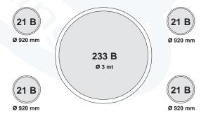
The propellant used has been heptane. Two fire tests have been performed, with extincion time of respectively 9 and 10 seconds; the test result was positive.
