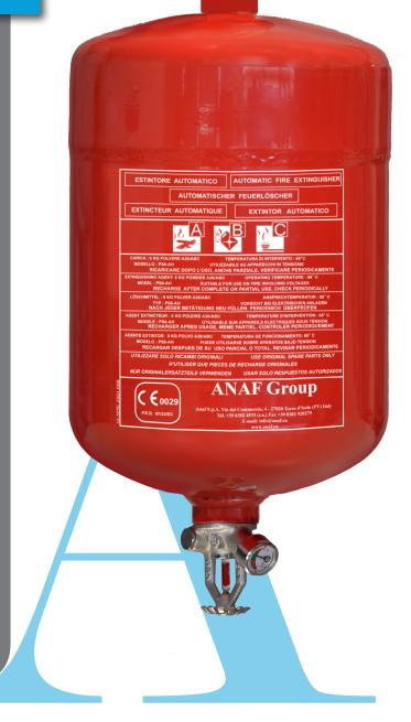
PS6-AT is an automatic pressurized powder fire extinguisher with pressure gauge. The activation temperature is 68 or 79 ° C. Certified to the Pressure Equipment Directive PED 97/23/EC. Capacity 6kg.
