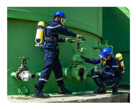
The Aeris Confort Type 2 is composed of a high/medium pressure (HP/MP) reducer, a comfortable harness with aramid fibre straps, a full-face mask, a positive pressure demand valve and an integrated alarm in the handle of the high pressure gauge.
